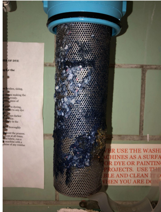
Lint-Luv-R filter screen after 10 loads, 4/5/22
