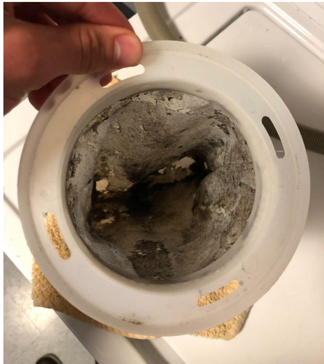
Filtrol filter bag after 20 loads, 4/21/22
