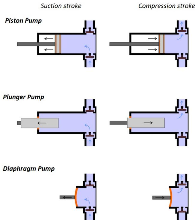
**Figure 2.** Basic mechanism of each of the three reciprocating pumps<sup>7</sup>.
