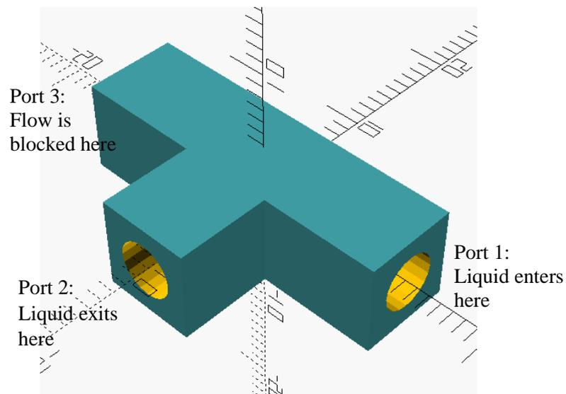
**Figure 6.** Check valve should result in a specific flow of liquid.
