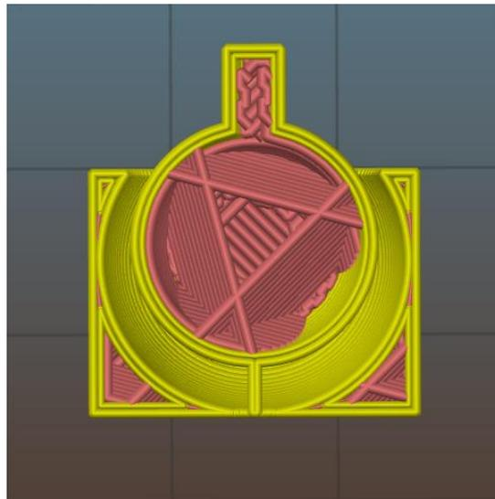
**Figure 4.** Cross section of initial design for the ball in socket. Dimensions: sphere—15 mm diameter, support pillar—1 mm diameter, spherical cavity—18 mm diameter, cube—20x20x15 mm. The handle on top was merely to help snap the ball off the support pillar.
