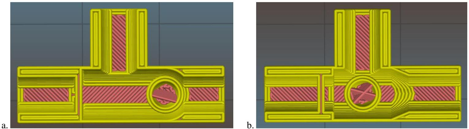
**Figure 7.** Cross section comparison of different valve designs. Figure a. is the original design with spherical cavity. Figure b. is updated design with conical cavity.
