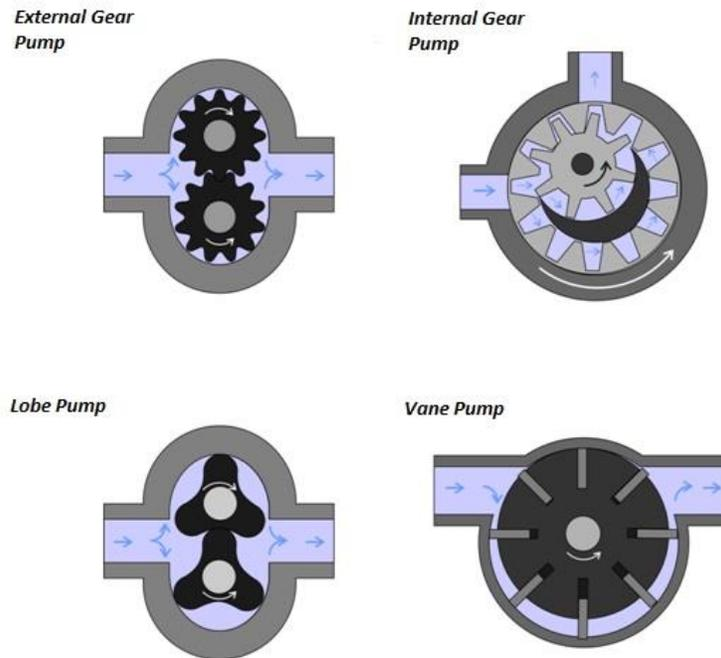
**Figure 3.** Design of rotary pumps. Each rotary pump contains a rotating element and a chamber which holds the fluid being pumped<sup>7</sup>.
