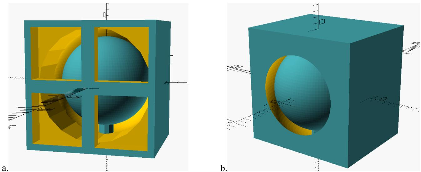
**Figure 5.** Initial valve design. **a.** This side of the valve permits flow; ball moves through a cylindrical channel and is kept in place by the cross. **b.** This side of the valve prohibits flow; ball becomes nestled in a spherical cavity, creating a seal.
