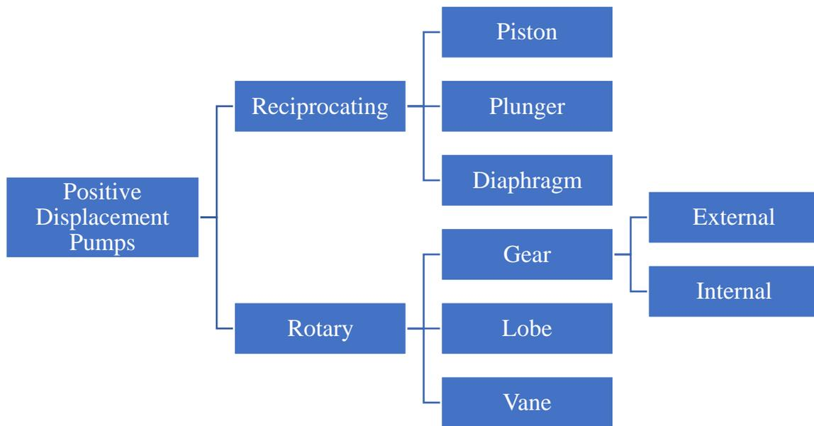
**Figure 1.** The reciprocating piston pump, which was the goal for this study, is only one of several types of positive displacement pumps.
