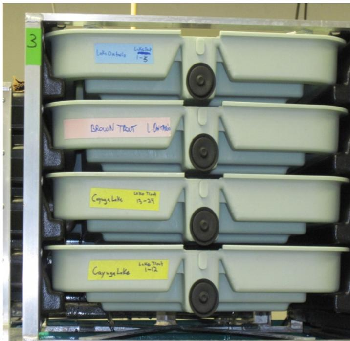
Figure 3. California hatching trays used for lake trout eggs incubation.
