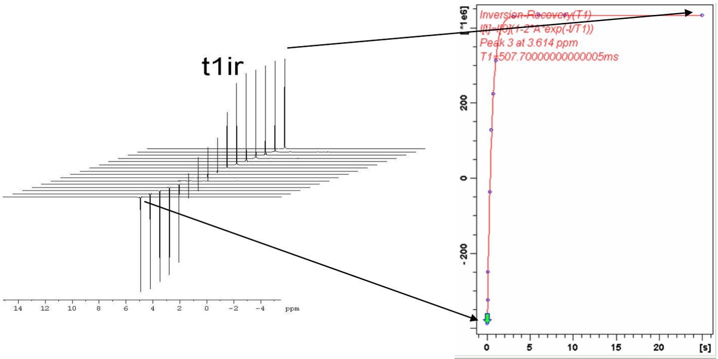
*Figure 10,  $T_1$  slices and  $T_1$  time constant plot*
