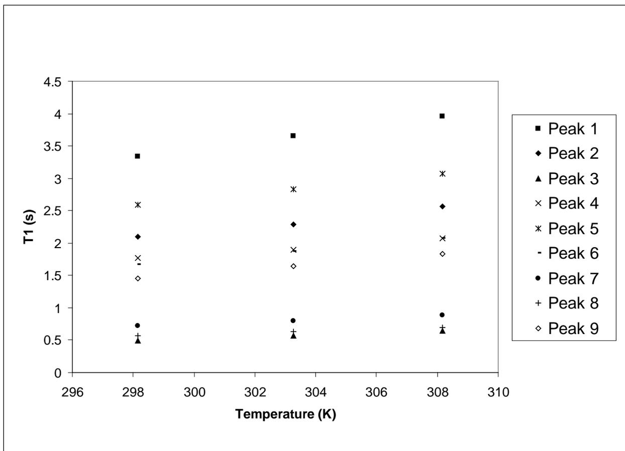
Figure 20b,  $T_1$  time constants for 3.5% by mass surfactant solutions containing D-limonene
