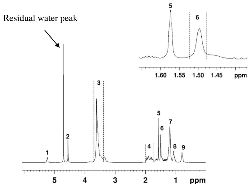
*Figure 18, sample  $T_1$  slice showing the signals for which  $T_1$  and  $T_2$  time constants were determined*
