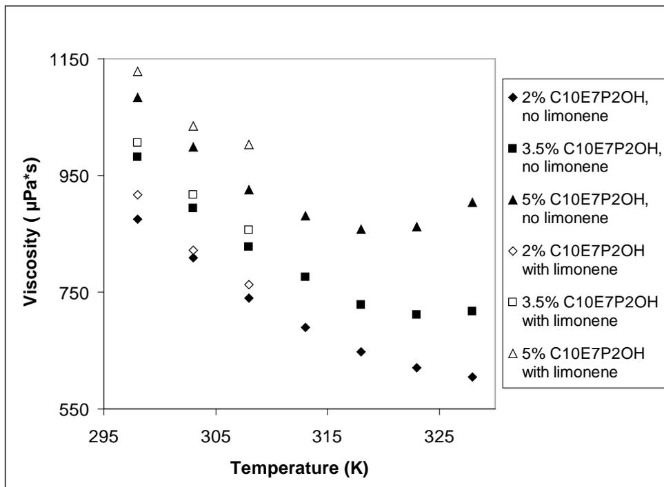
Figure 15, Viscosity of C10E7P2OH solutions at various temperatures
