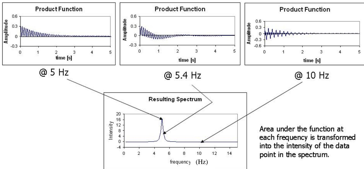
*Figure 8, Conversion of the product functions to the final spectrum*
