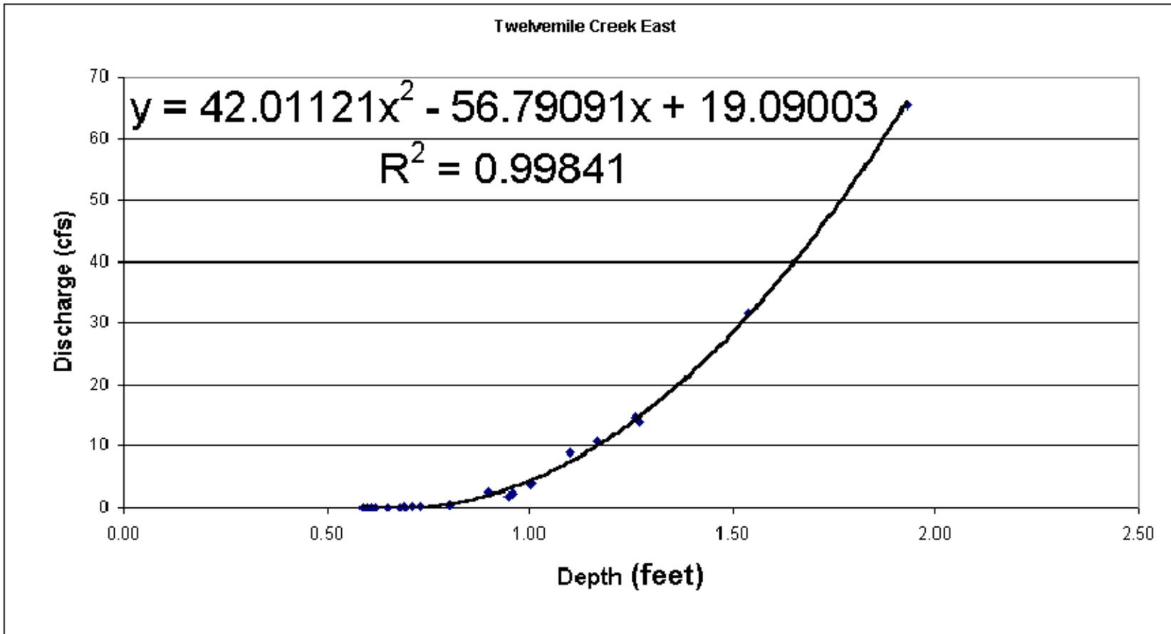
Figure 2. Rating curve for Twelvemile Creek East to be used for creek depths less than 2 feet.
