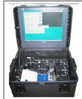
**Figure 3a. FlowCAM II fluid imaging system**
