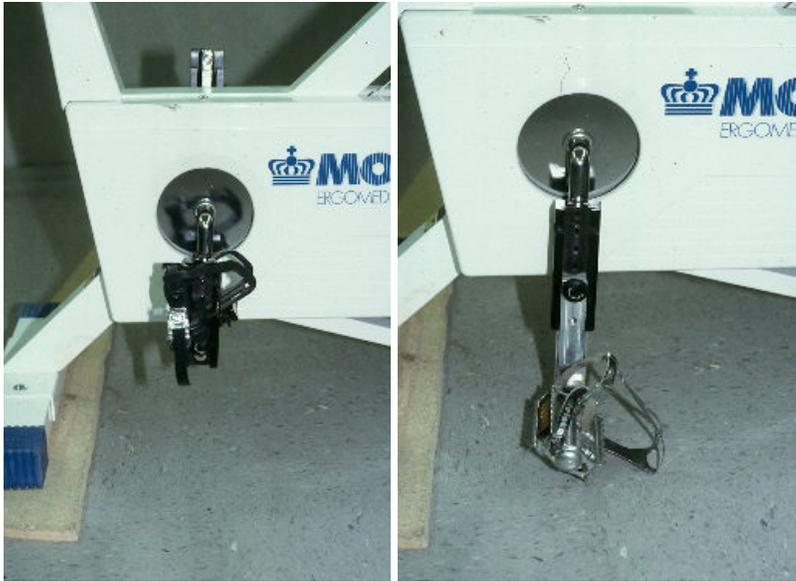
Figure 2: Adjustable pedal shaft mechanism and cranks
