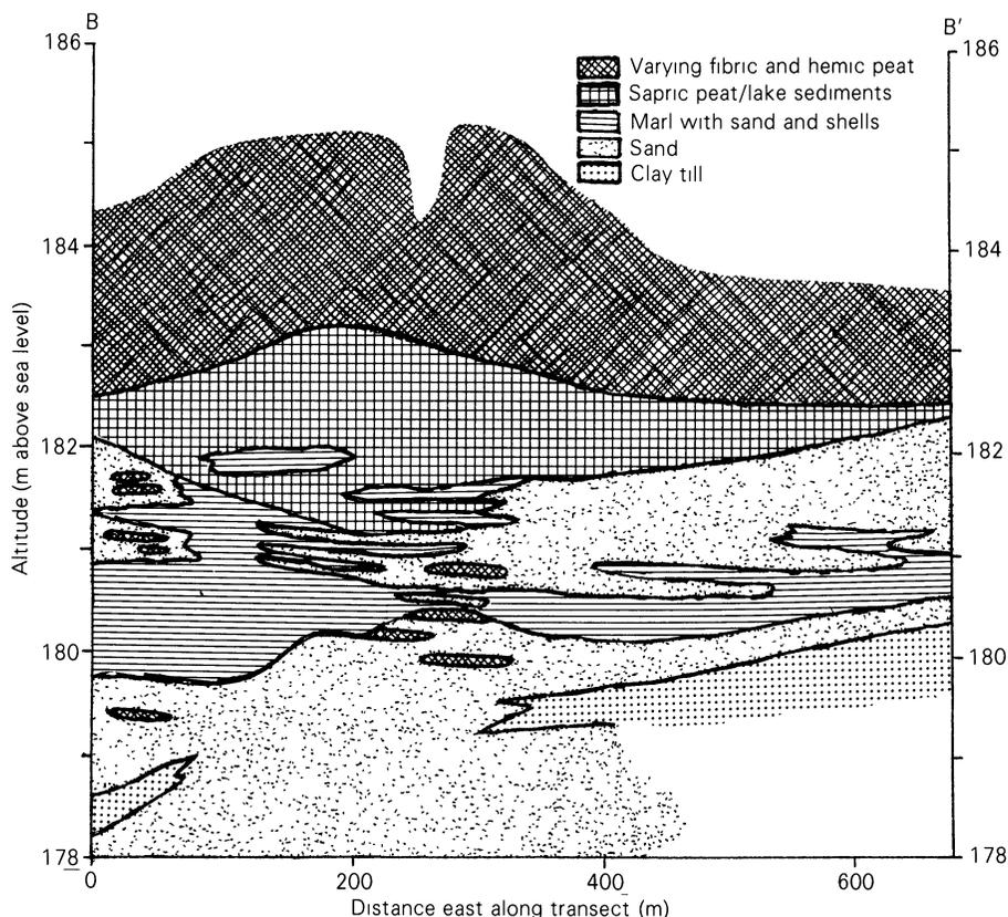
FIG. 5. East-west stratigraphic cross-section of Cowles Bog Wetland Complex across mound. (From vibra-core descriptions.) Line of transect (B-B') is shown in Fig. 1. The vertical exaggeration is  $\times 80$ .
