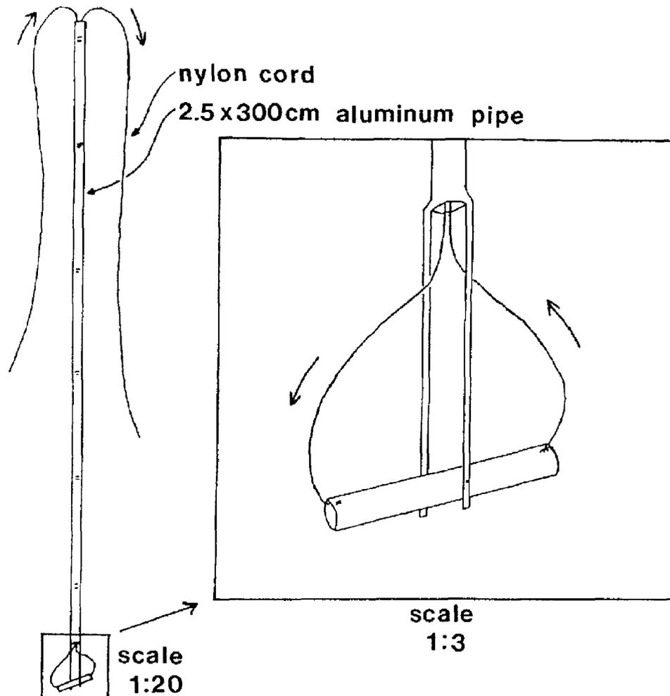
Figure 2. Bog mat depth sampler, which is inserted into core hole, opened into an inverted T, and lifted until resistance is met.
