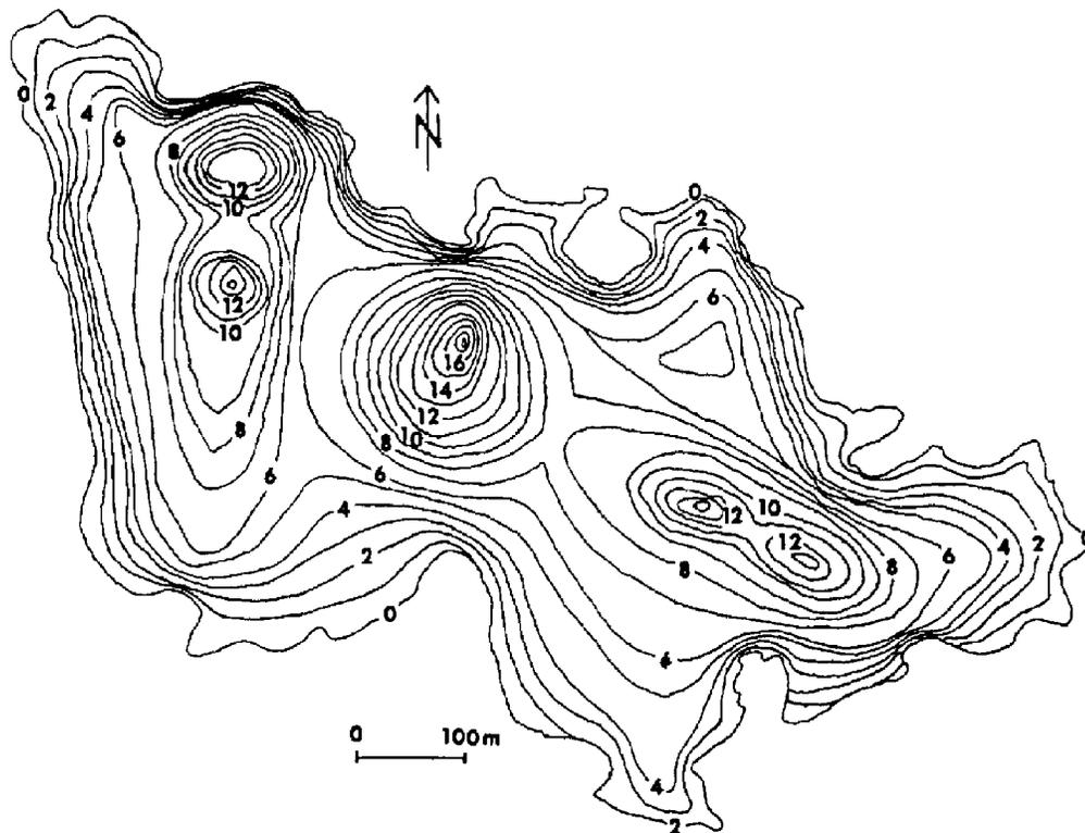
Figure 3. Topographic map of Pinhook Bog basin, the surface of the glacial till (clay). Contour interval is 1 m. The clay does not come to the surface at some locations along the southern boundary of the bog.
