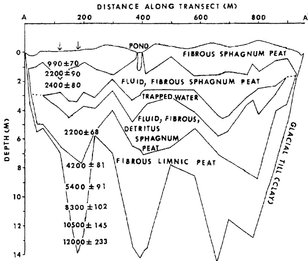
Figure 4. Stratigraphic cross-section of Pinhook Bog along transect A-A' (see Figure 1) with radiocarbon dates at sites 120 m and 180 m. The vertical exaggeration is X 50.
