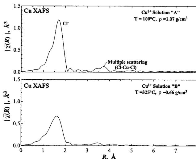
FIG. 5. The  $|\tilde{\chi}(R)|$  plots from the magnitude of the Fourier transform of the  $\chi(k)$  spectra shown in Fig. 4. This  $|\tilde{\chi}(R)|$  plot is uncorrected for phase shifts whereas the actual distances are reported in Table II.
