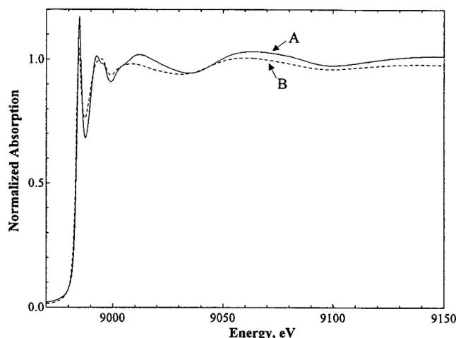
FIG. 3. X-ray absorption spectra at the Cu  $K$ -edge for two solutions corresponding to locations marked in the images in Fig. 2 and the starting compositions reported in Table I. The two spectra were scaled to a common edge height.
