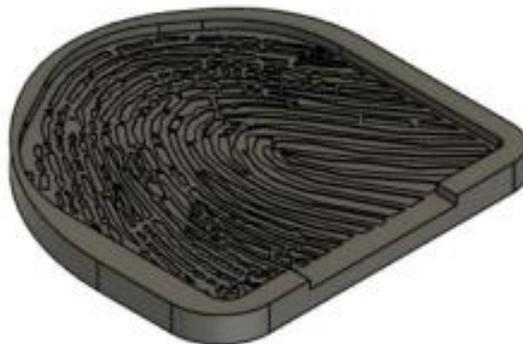
Figure 4 – The manually modeled fingerprint mold
