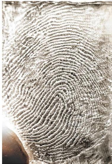
Figure 12 – Indirect Collection Copy – result of using Selva3D to create a direct copy of the original fingerprint based on the indirectly collected base (with 50 micron ridge spacing)
