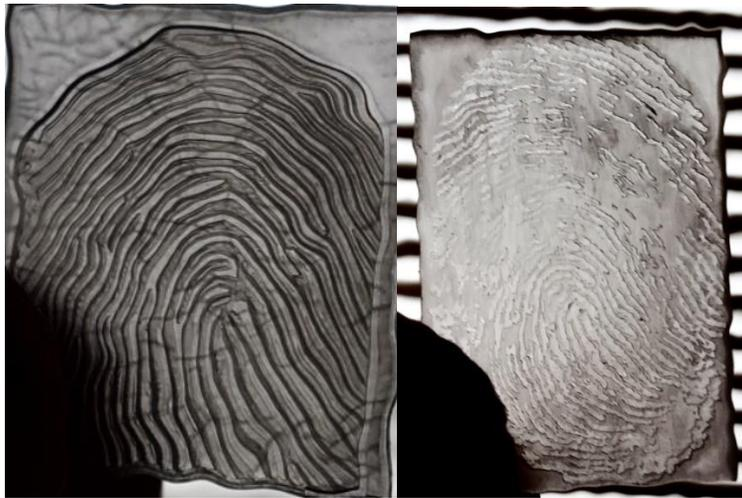
Figure 11 – Indirect Collection Mold – the manually constructed model (left) and the automatic Selva3D model (right), both with 50 micron ridge spacing
