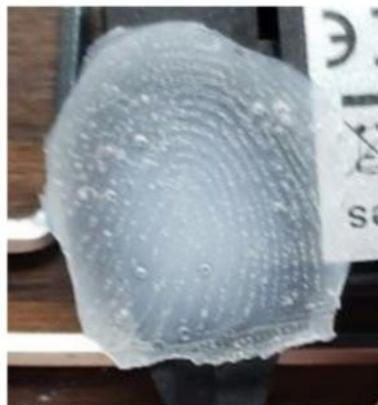
Figure 8 – The fabric glue cast of the fingerprint (as taken from the 3D printed mold)
