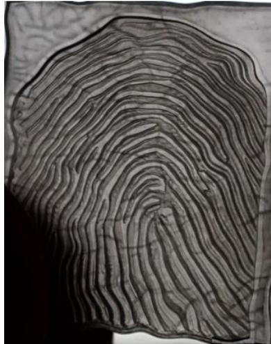
Figure 10 – The manually constructed mold printed on an SLA printer with 100% scaling
