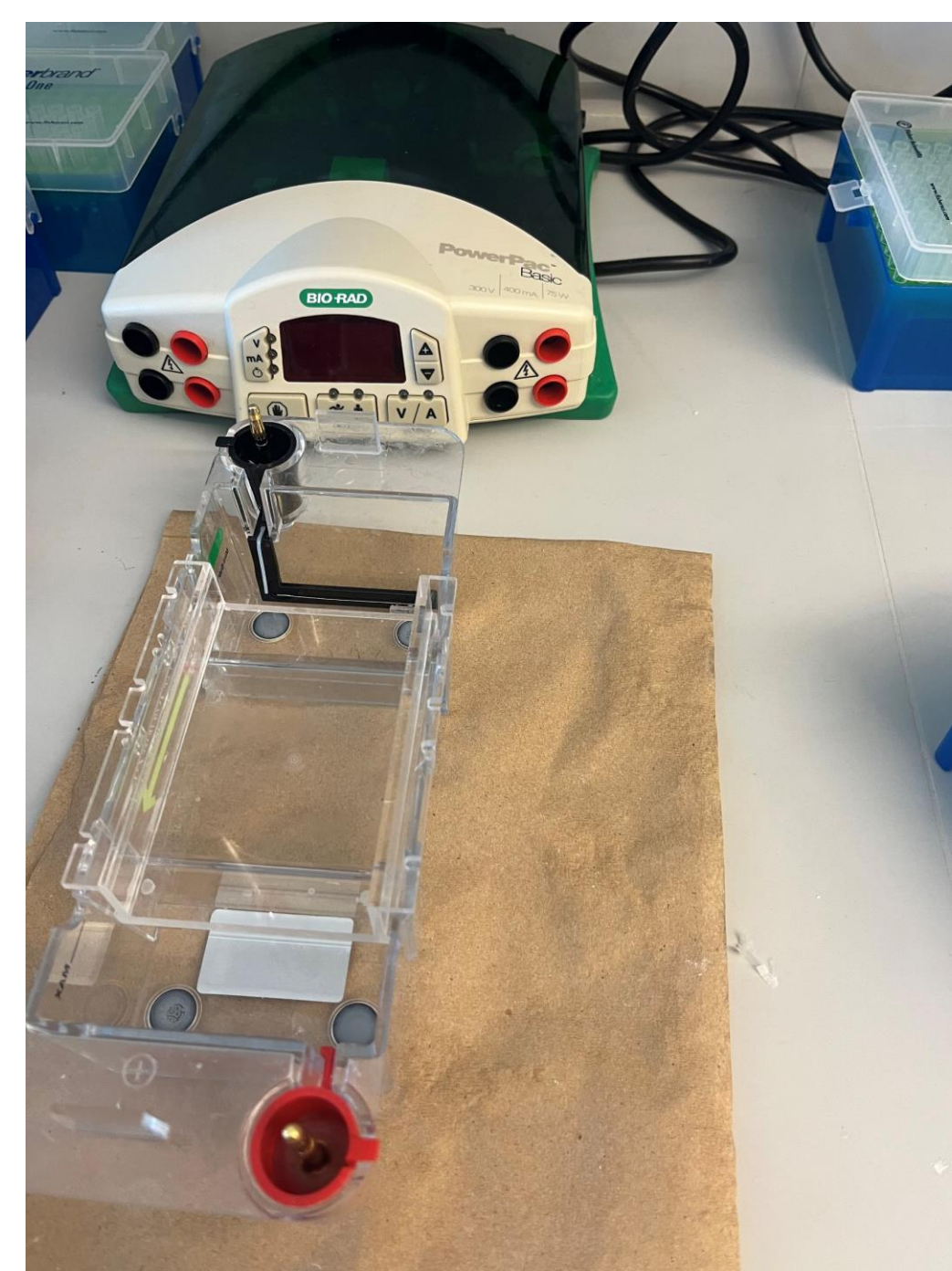
Electrophoresis chamber and power supply. After the gel has been set, it can be placed in the chamber and submerged in 1x TAE buffer before running.
