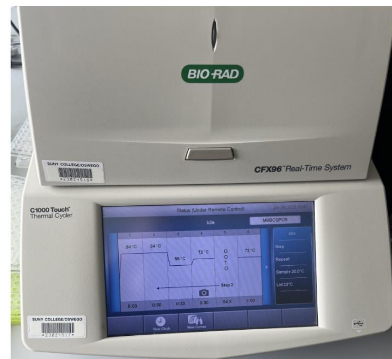
CFX96 real-time system C-1000 thermal cycler: used to gather real-time amplification data as well as the melting curve.
