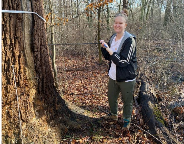
Image 2; Obtaining core sample using 32-inch Haglof Incremental Borer. Note the scarring on the right side of the tree.
