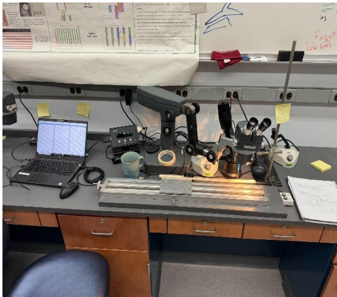
Image 4; Velmex Tree Measuring System set up to collect data on a core sample.
