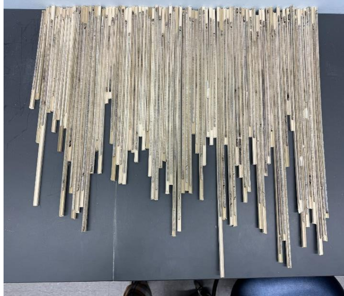
Image 5; All mounted and sanded core samples.
