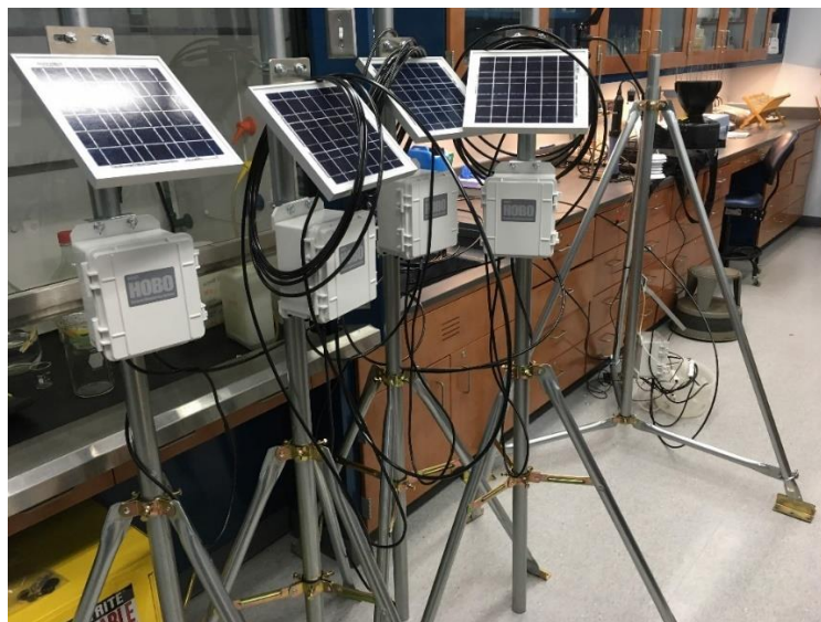
Figure 5. Tripod set up with mounted solar panels and HOBO RX3000 data loggers.
