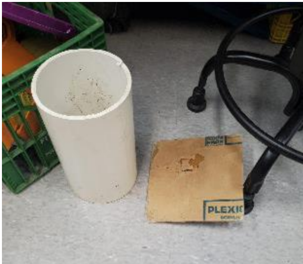
Figure 3. The plexiglass sheet and PVC pipe used to collect the sand from the beaches.
