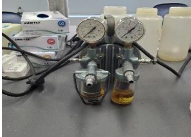
Figure 5. The vacuum filter extractor used.
