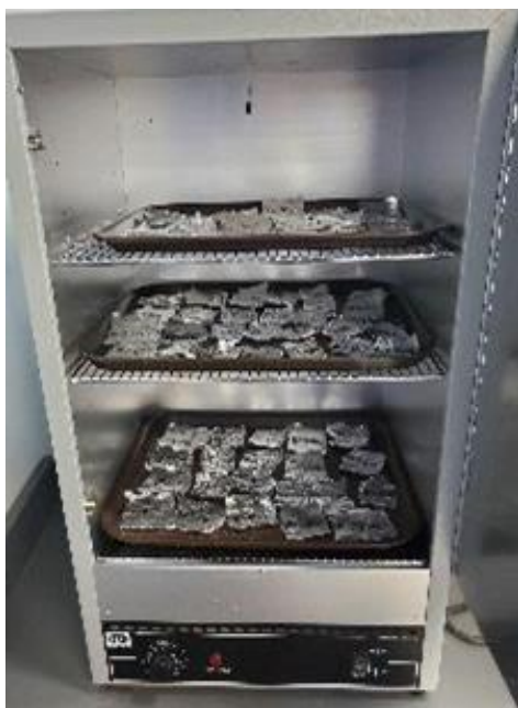
Figure 6. Tinfoil, with microplastic filters inside drying in a lab oven.
