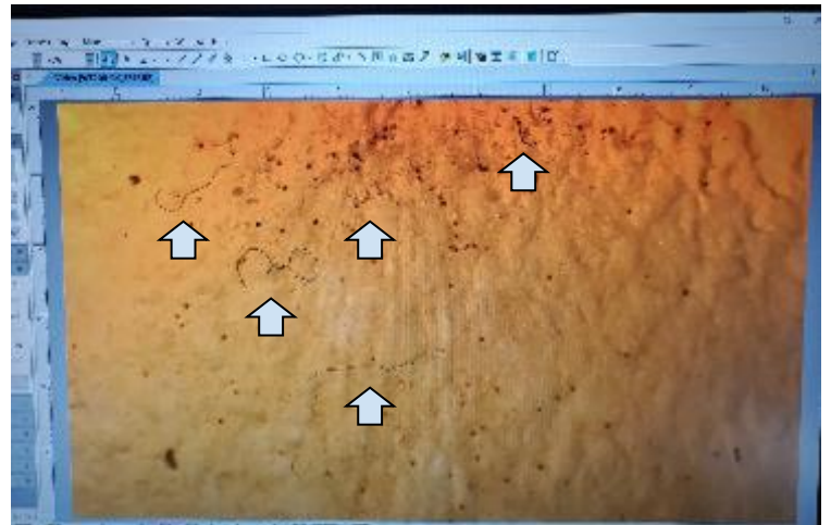
Figure 9. Example of filter from Read Sanctuary. Multiple microplastics shown, with the majority being filaments, shown by arrows.
