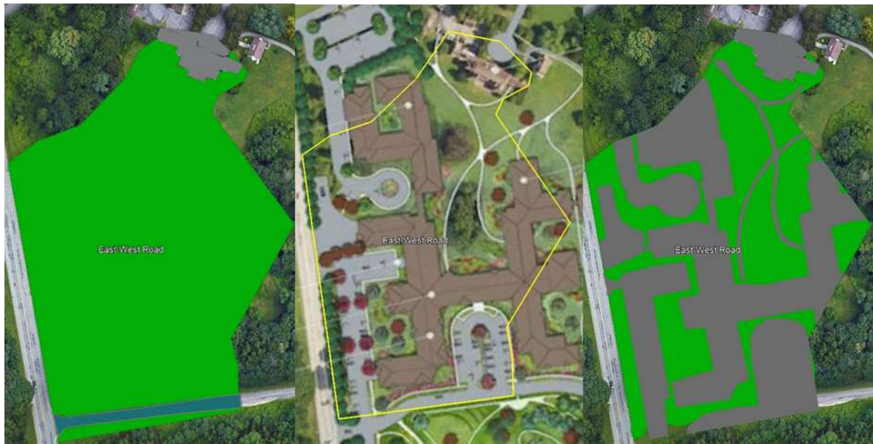
Figure 18 Current East-West Road conditions vs. future changes in land use and impervious surface. Green= vegetated areas, gray/blue= impervious surface
