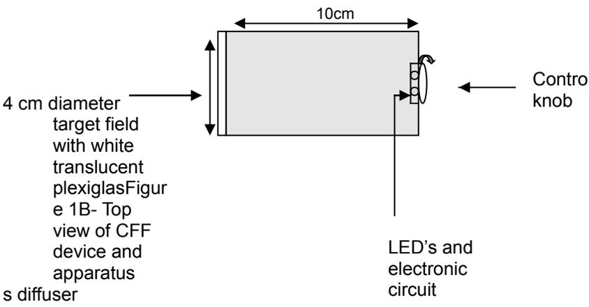
Figure 1B- Top view of CFF device and apparatus
